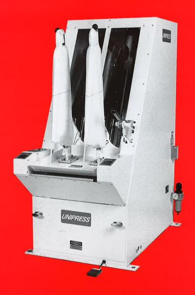
The ABS Air Bag Sleever produces top quality fully pressed sleeves of all sizes and shapes in one operation. Contoured chests, non-porous air bags and automatic measuring ensure high quality uniformly finished sleeves. The non-porous air bags are inflated with compressed air and act as malleable expander blades which expand to the contour of a wide range of shirt sleeves. The pressurized air bags fit precisely into the highly polished contoured chests,
