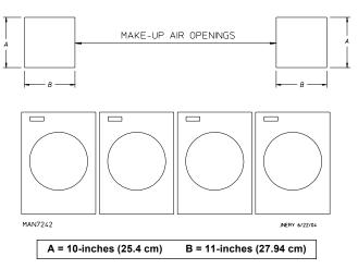
EXAMPLE: For a bank of 4 M31SL dryers, 2 unrestricted openings measuring 10-inches by 11-inches (25.4 cm by 27.94 cm) are acceptable.
