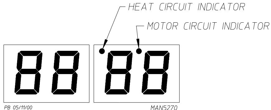
The L.E.D. indicator dots located at the top portion of the display indicates the various microprocessor controller (computer) output functions while a cycle is in progress. These dots **DO NOT** necessarily mean that the outputs are functioning. They are only indicating that the function (output) **should be** active (on).
