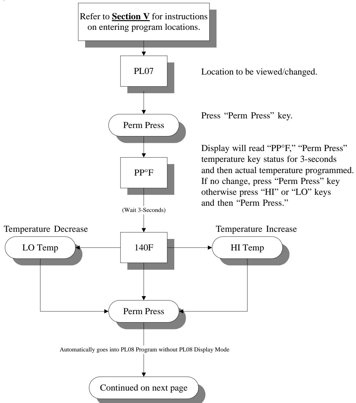
Summary: Perm press temperature is programmable from a minimum of 100° F to a maximum of 160° F in ten-degree increments or from a minimum of 38° C to a maximum of 71° C in five-degree increments.
