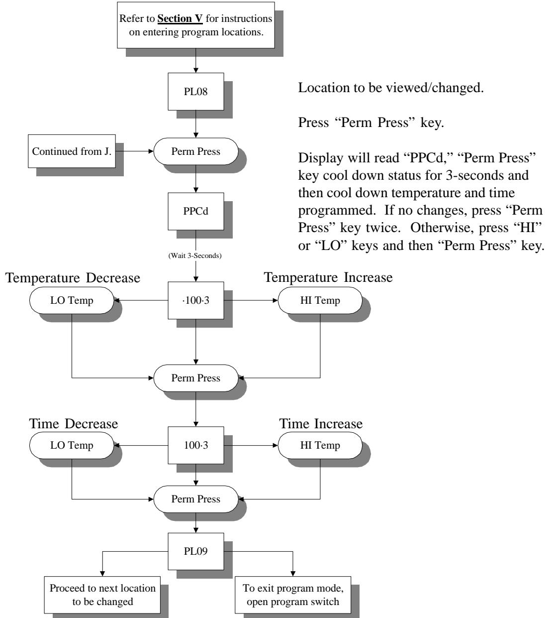
Summary: Cool down temperature is programmable from a minimum of 100° F to a maximum of 160° F in ten-degree increments or from a minimum of 38° C to a maximum of 71° C in five-degree increments.
