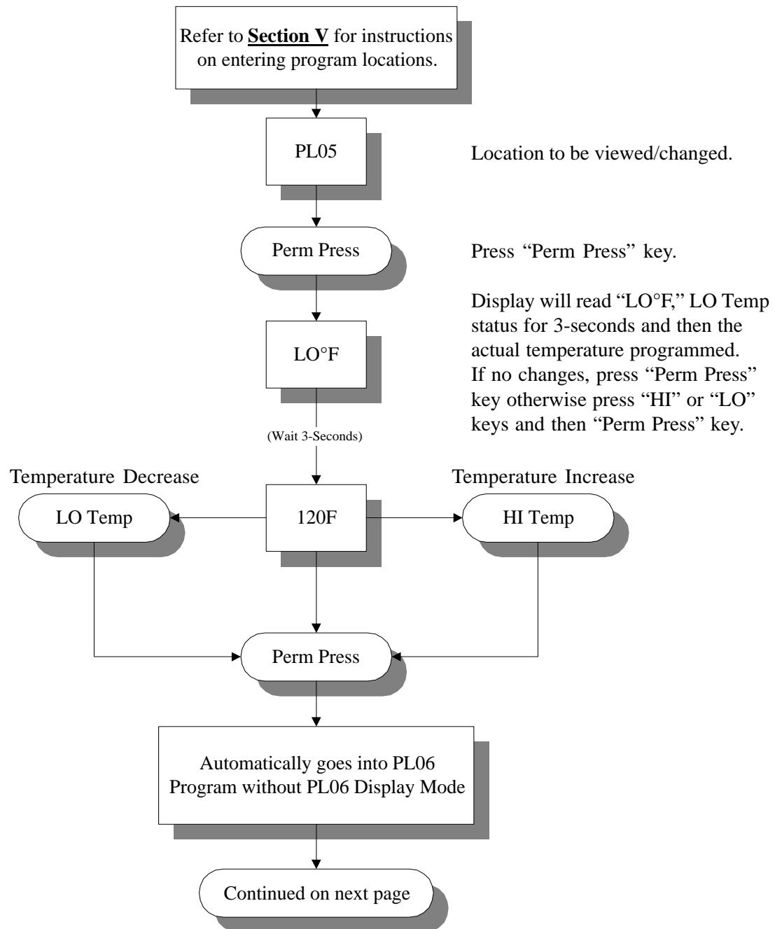
Summary: Low (LO) temperature is programmable from a minimum of 100° F to a maximum of 160° F in ten-degree increments or from a minimum of 38° C to a maximum of 71° C in five-degree increments.
