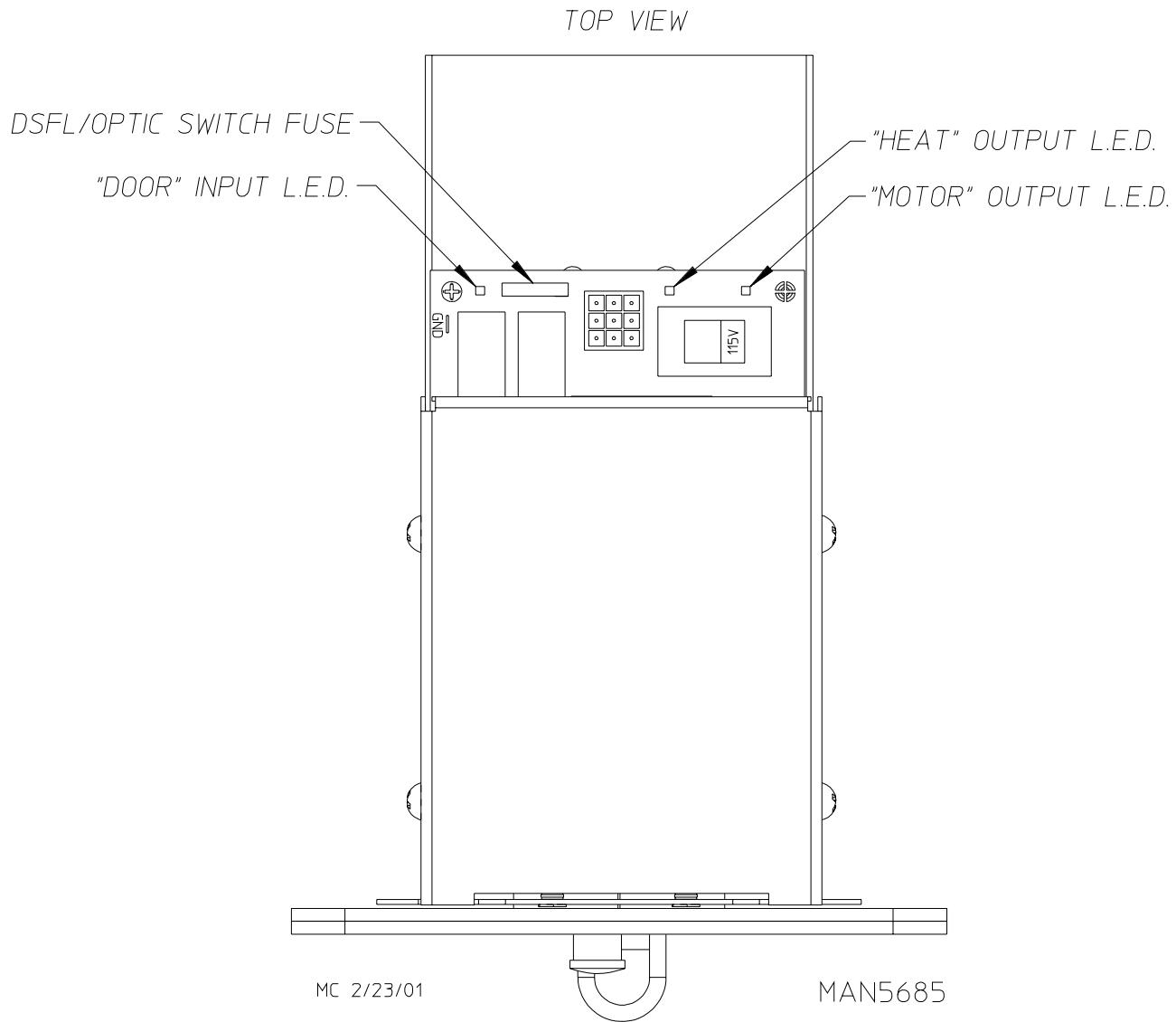
There are three (3) light emitting diode (L.E.D.) indicators ("red" lights) located on the top of the microprocessor controller (computer), which are identified/labeled as "DOOR," "HEAT," and "MTR" (motor). These L.E.D.s indicate that the outputs of the microprocessor controller (computer), or in the case of the door switch, the inputs are functioning.
