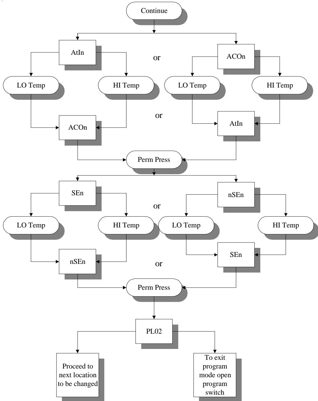
Display will read coin/time accumulation status. I.E. "AtIn" accumulative time or "ACOn" accumulative coin. If no change, press "Perm Press" key, otherwise press "HI" or "LO" keys and then press "Perm Press" key.
