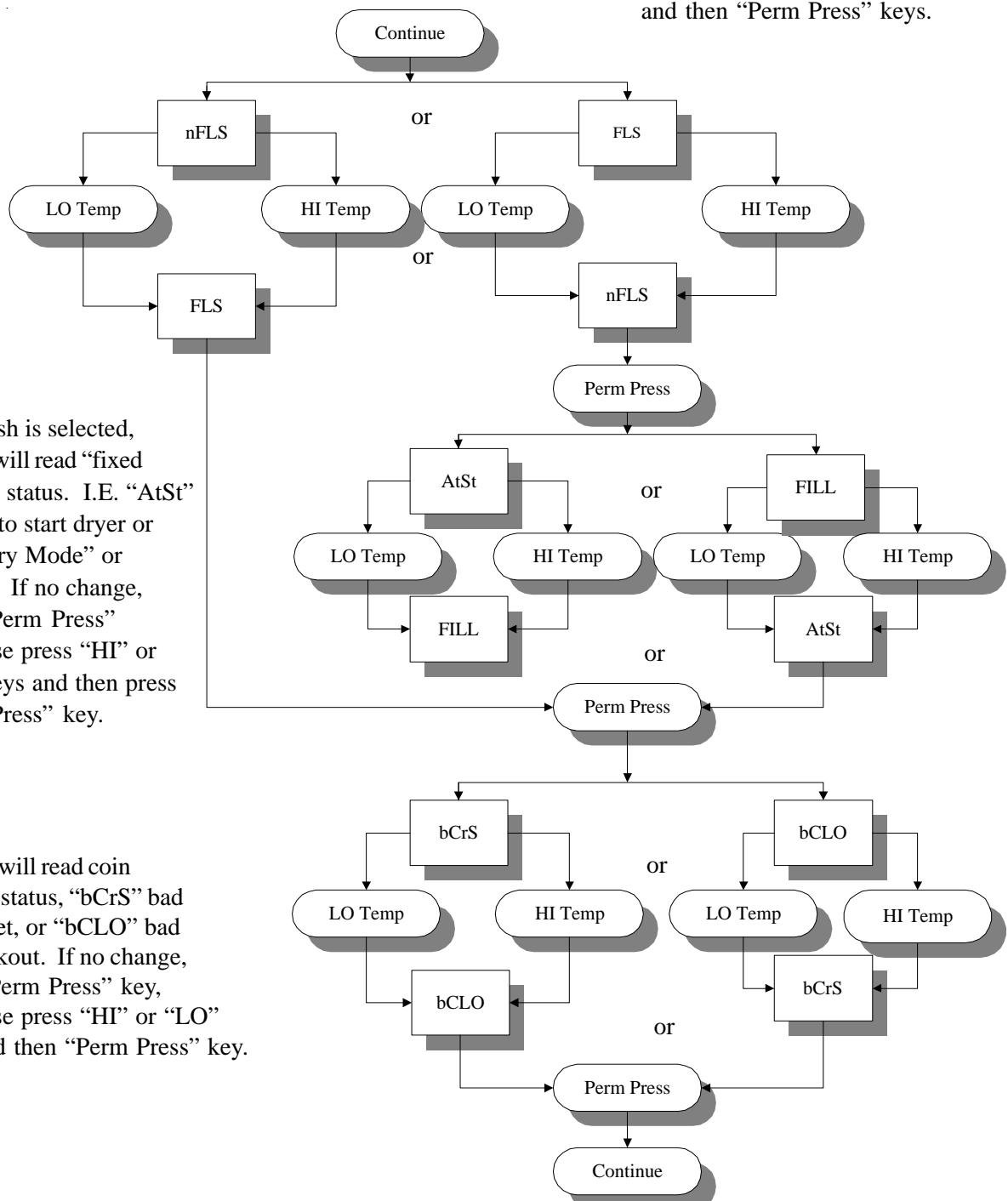
If no flash is selected, display will read “fixed display” status. I.E. “AtSt” amount to start dryer or “Free Dry Mode” or “FILL.” If no change, press “Perm Press” otherwise press “HI” or “LO” keys and then press “Perm Press” key.
