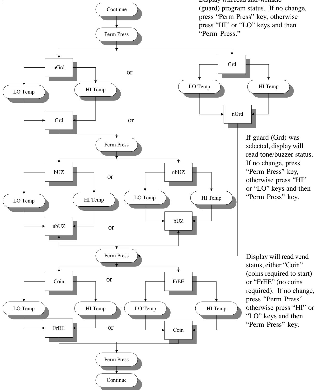
Display will read light emitting diode (L.E.D.) display status. Either no flash (nFLS) or flash (FLS). If no change, press “Perm Press” key, otherwise press “HI” or “LO” keys and then “Perm Press” keys.
